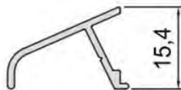
KOD-CODE AC-5578-15 TEORİK AĞIRLIK THEORETICAL WEIGHT 0,136 Kg/m
